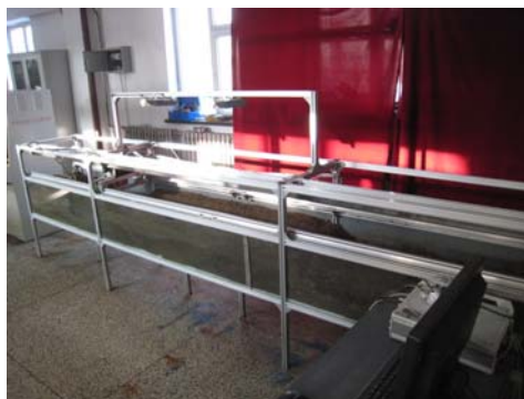
Figure 1. The experiment table of the small glass soil bin.
